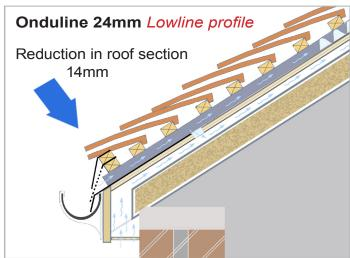
So now the choice is yours select either the existing proven Ondutile; or the new Ondutile Lowline profile base sheet to suit your roofing design requirements. Allowing roofing tiles and slates to be laid below the manufacturers minimum recommended roof pitch with confidence.
