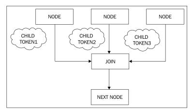
When all the child tokens arrive at the join node, the child token (subpaths of execution) is marked as ended. It automatically triggers a signal to the root token to continue.
