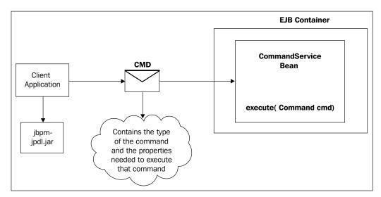
As you can see in the figure, the client application will create and send a command to the CommandServiceBean to be executed. Each command will be of different type, depending on its behavior, and it will contain different properties to be executed.
