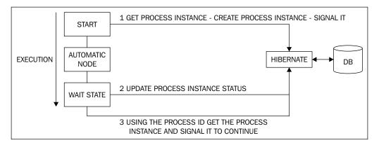
In this case, the third step can be done by the other decoupled thread, which restores the process status using the process ID and then signals it to continue the execution.
