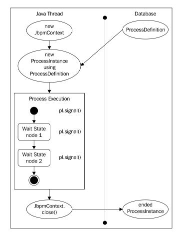
This image represents the behavior of the first block of code described previously. We can see how our process is executed from start to end, by only interacting with the database to get the ProcessDefinition that needs to be deployed previously, and to persist the ProcessInstance that has already ended. This last interaction with the database will let us see that the process has successfully executed from start to end.
