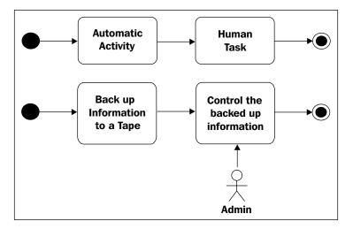
This process is just a simple tape backup process. This process will start and execute a tape backup (that is just an automatic activity). Imagine this process needs to be executed each night and it must finish before the employees enter the company in the morning.
