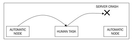
Our process is running in memory, and an actor finishes a human task and this task completion will trigger a signal that will take the transition to the next node. What happens, and what is supposed to happen if the server shuts down in the middle?
