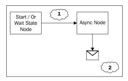
If the server crashes at stage 1 (and the previous node is not marked as an async node), we must manually execute the signal() method again, in the previous node, to continue or restart the execution. This means that we will lose the activities executed after the last wait state.
