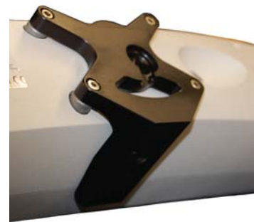
Mounting Bracket fitted to Position Sensor
