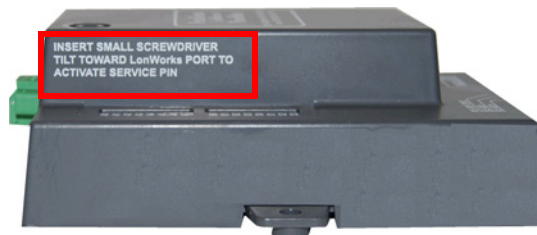
Figure 2.12: Location of ProtoCom-Lon Service Pin Instructions
