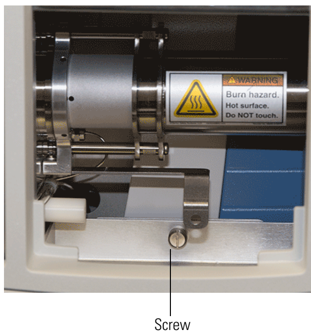
Figure 8-39. Locating the Back Screw
