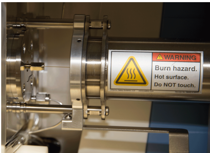
Figure 6-17. Correctly Installed Column in MS Transfer Line
