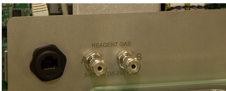
Figure 5-8. Connecting the CI gas supply
