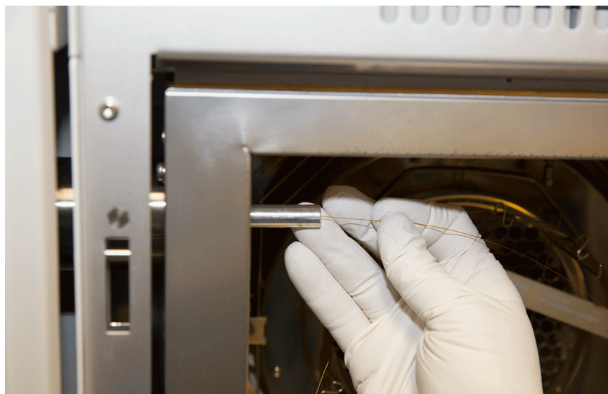
Figure 6-10. Inserting the New Column through the GC Transfer Line
