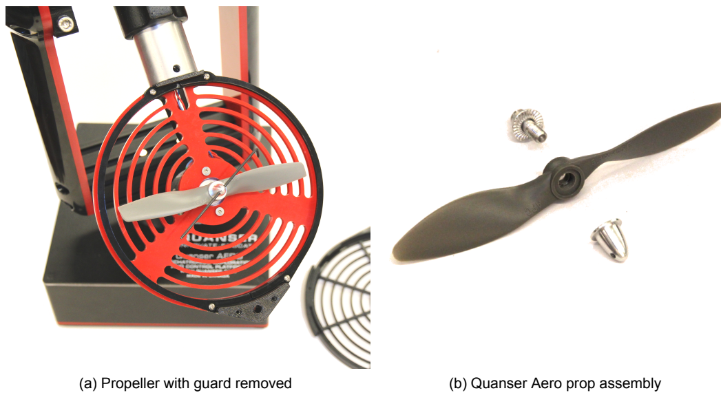
Figure 3.3: Quanser Aero propeller change steps
