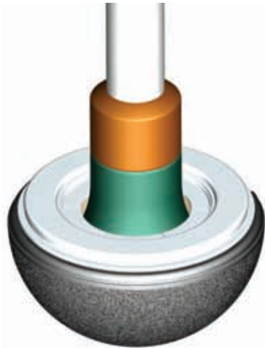
Alignment ring allows for easy placement of the hard bearing liner in the shell. The liner impactor can then be inserted through an opening in the alignment ring and the liner can be seated with an impaction force.
