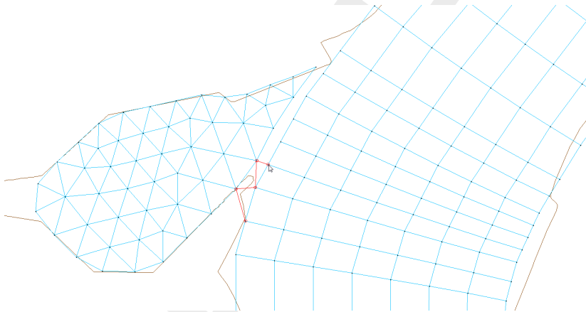
Figure 6.19: Coupling of the two grids (regular and irregular, in blue) through manually inserting connecting grid lines (in red lines) between the two grids.
