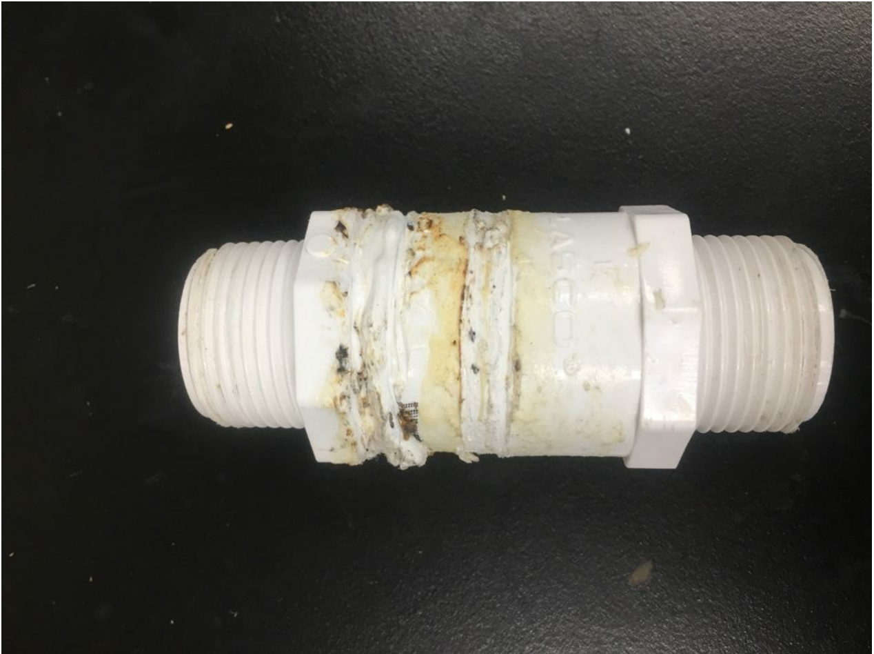
Figure 3: Spring 2018 Fabricated Male to Male PVC fitting. This is the current team's fitting fabricated in Spring 2018, where you can see the welds done with the hand held PVC welder.
