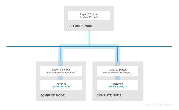
In order to allow instances on separate nodes to communicate as if they're on the same logical network, you'll need to use an encapsulation tunnel such as VXLAN or GRE. It is recommended you consider adjusting the MTU size from end-to-end in order to accommodate the additional bits required for the tunnel header, otherwise network performance can be negatively impacted as a result of fragmentation. For more information, see *Configure MTU Settings*.
