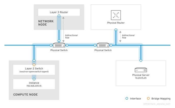
Inconsistent MTU values can result in several network issues, the most common being random packet loss that results in connection drops and slow network performance. Such issues are problematic to troubleshoot, since every possible network point needs to be identified and examined to ensure it has the correct MTU value set.
