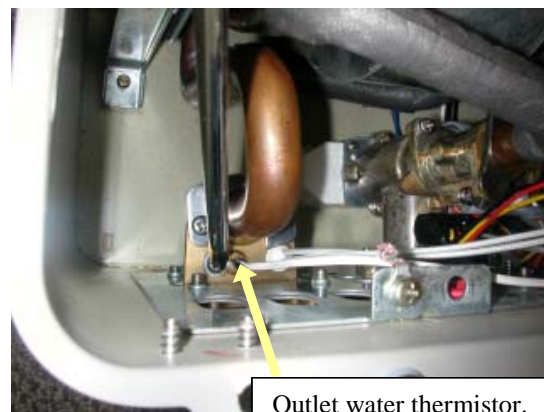
Outlet water thermistor.
