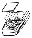
The battery compartment is found at the back of instrument. To open the battery compartment, push in the direction of the arrow and lift up the cover. Note the polarity of the battery before inserting it into position. After replacement, place the cover back and press down until it locks tight.
