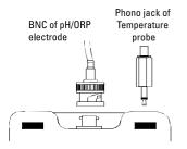
To connect the electrode into meter, align the connector slots with the posts of meter's socket and rotate the connector clockwise until it locks. Do not force when connecting. To remove, simply rotate the connector in anti-clockwise direction until it unlocks, and slide the connector off the socket.
