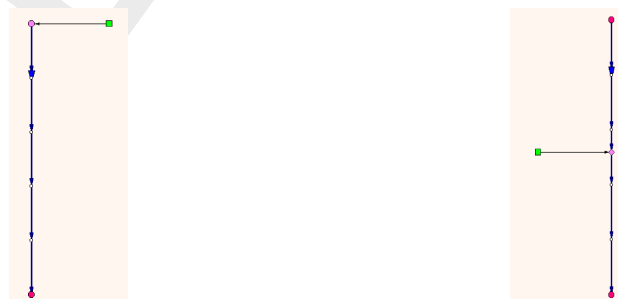
Figure 5.195: Two ways to connect an RR Unpaved node to a channel (only available if you have a license for the flow module).
