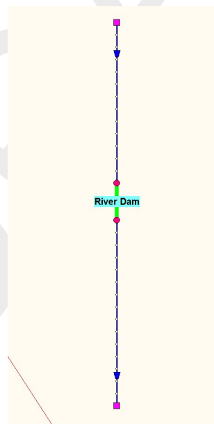
Figure 5.218: Bbranching of a 1D river dam using a "Flow 1D Dam Break Branch"
