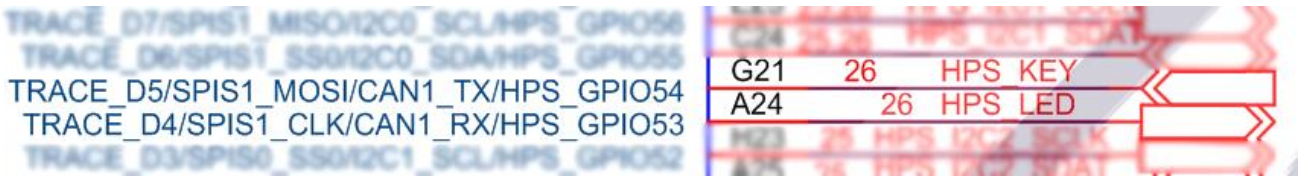
Figure 9-5. HPS_KEY_N & HPS_LED on DE1-SoC Schematic. Note that the schematic uses “HPS_KEY” instead of “HPS_KEY_N” as the name of the signal. This is a mistake, as the button is active-low, so the “_N” in the name is warranted for clarity.
