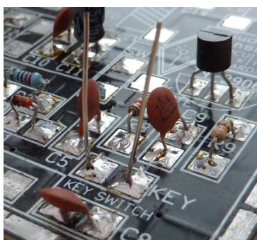
Now remove the insulation completely from two 2cm pieces of the black wire, and solder one end of each piece of bare wire to the KEY pads on the main board. Be careful you don't catch your fingers on these when they are stuck up in the air!
