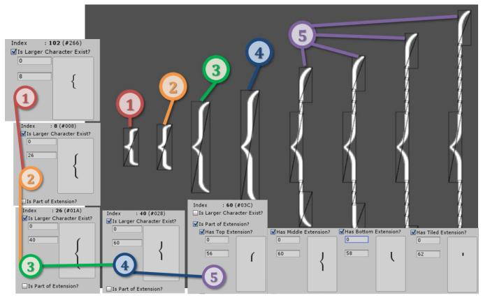
The idea is simple. This image shows every "level" and each "relation" character configuration of a delimiter \lbrace, which we note on each level in a number. \lbrace has up to 5 levels height. In the first level, a character with hash #266 holds the \lbrace symbol definition, and does refer to a larger character located in #008. So if #266 doesn't have sufficient height, the
