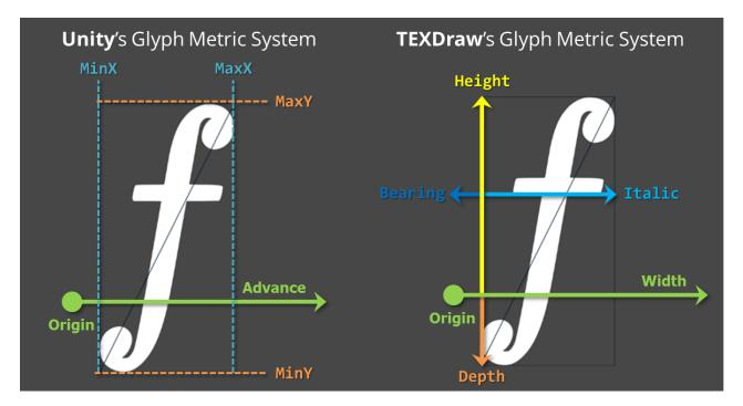
A character has a baseline (marked as green line), top and low bound. The image above will help you to understand each config which we will discuss below: (We provide each config explanation with relevant image and indicator colors)
