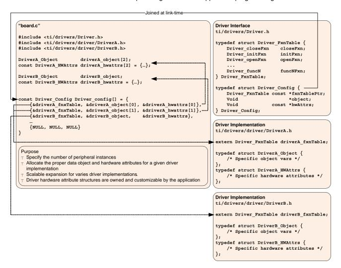
This diagram shows the relationship between a driver interface and two driver implementations. The driver interface named "Driver" is configured to operate on two driver implementations: "DriverA" and "DriverB". The driver's Driver\_config[] structure contains three instances. The first two instances are of type "DriverA" and the third is of type "DriverB".
