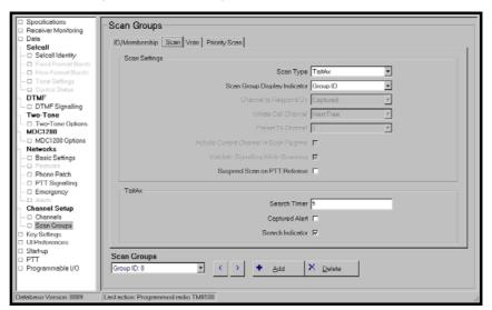
The objective of TaitAx as a Scan type is to utilise all channels (repeaters) in the area equally by ensuring users are accessing the next repeater.
