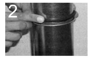
2. Place the harder black o-ring seal against the outside of the inner grey seal.
