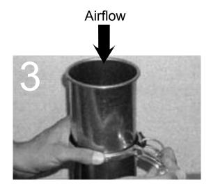
3. Finally clamp the standard Q-F clamp over the rolled metal edge of the adjustable nipple and the hard rolled black o-ring for a leak-free connection. [Make sure both seals fit completely under the clamp and that the air-flows from the cut pipe towards the adjustable nipple].
