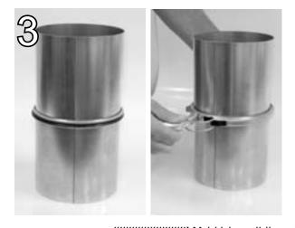
3) Join the gasketed end of the pipe to a non-gasketed end of the next part in the ducting run using a standard Q-F clamp. The oil-mist gasket, in addition to the gasket inside the Q-F clamp, provides dual protection against leakage.
