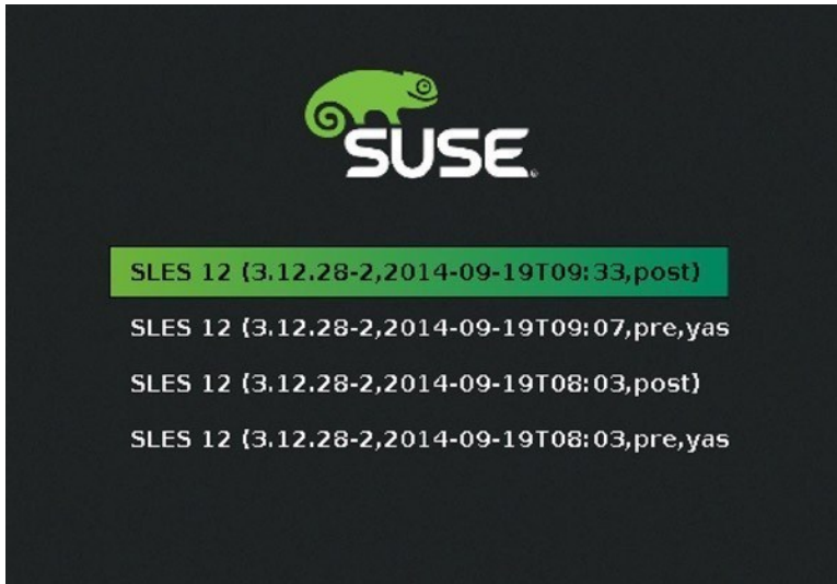
Figure 8-7. Reverting to a previous state by selecting a snapshot
