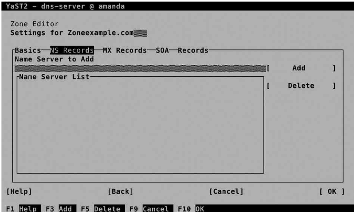
Figure 11-8. Configuring the name servers for a domain
