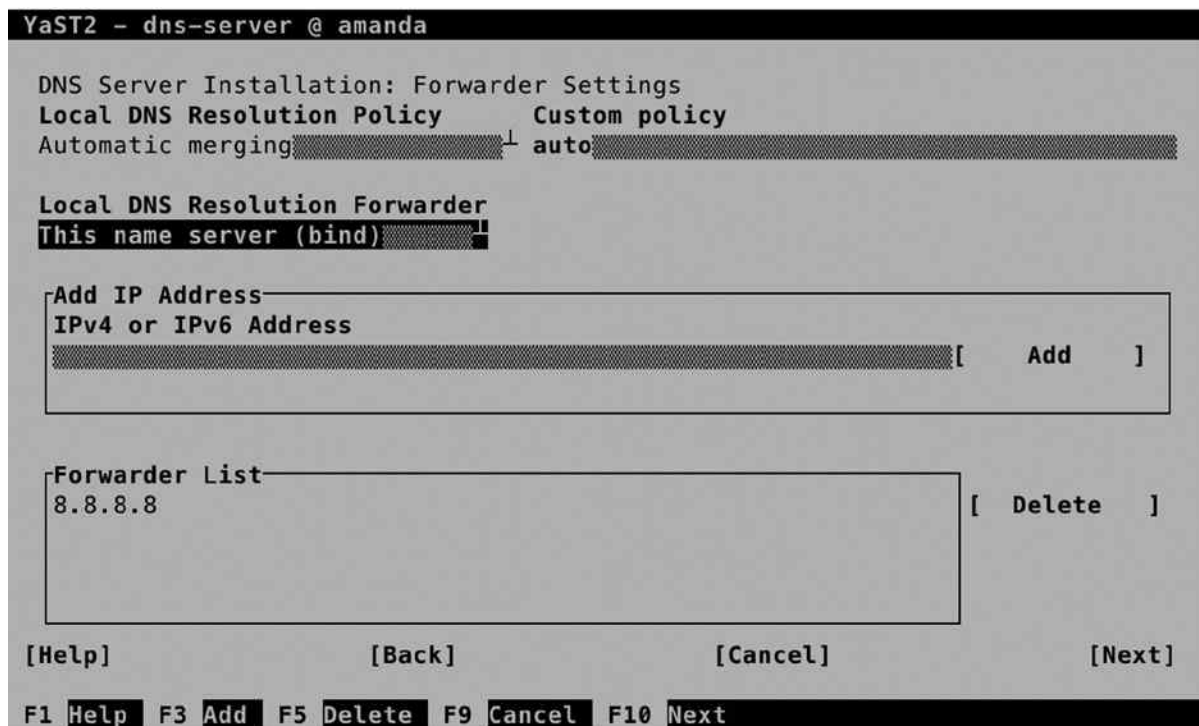
Figure 11-5. DNS forwarder configuration
