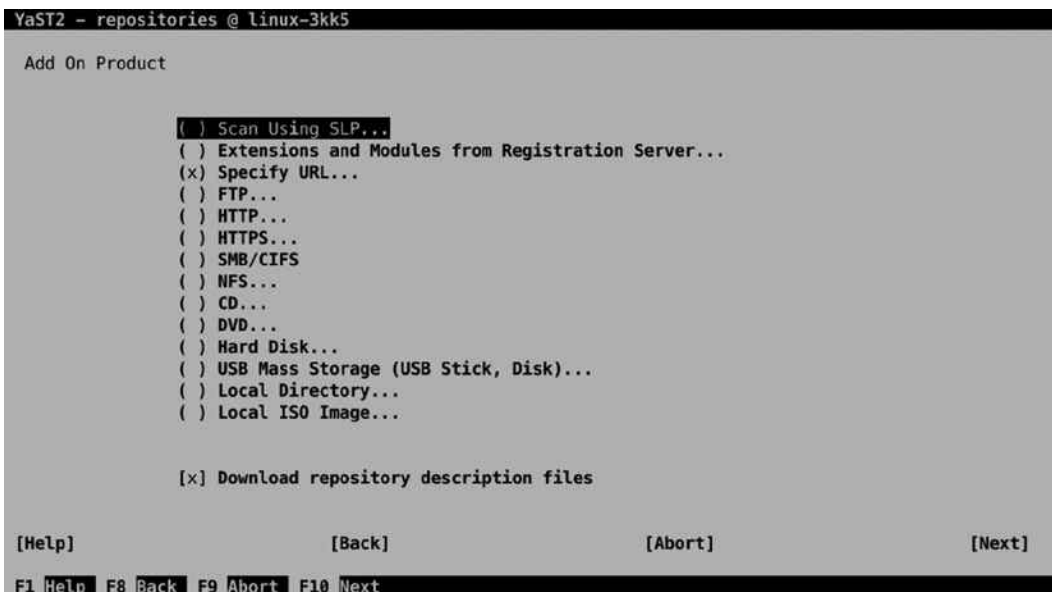
Figure 5-3. Selecting the source for the new repository
