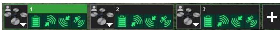
Image 17. Displaying three properly connected vehicles in UgCS with good telemetry status of all sensors
