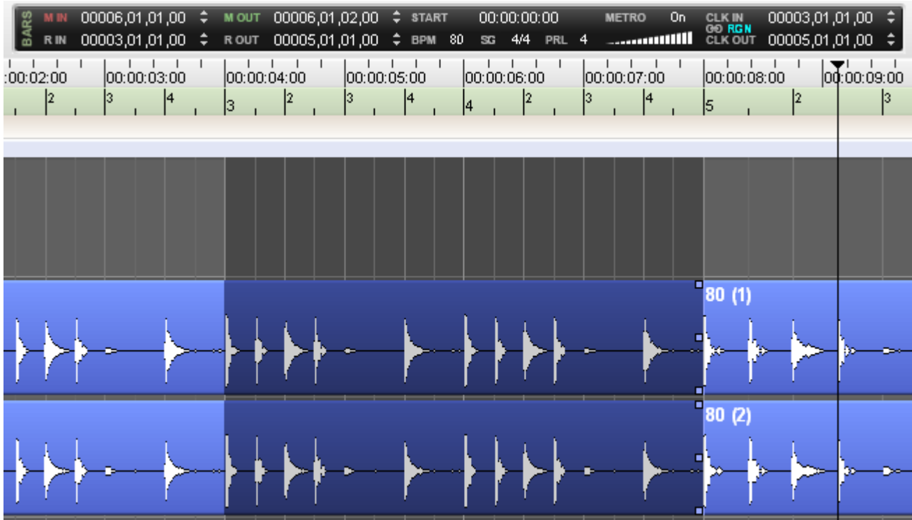
Metronome set at Region Selection Start and End time, using a 4 beat Pre Roll value.
