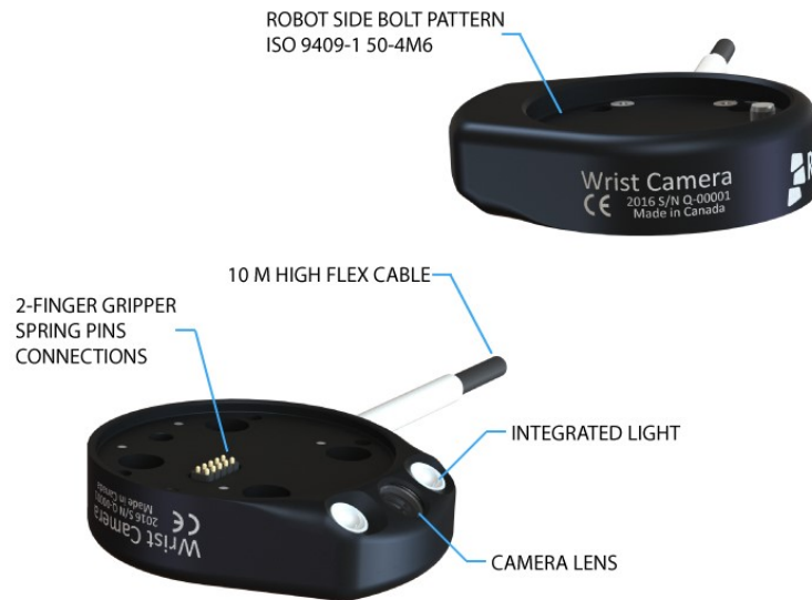
Fig. 1-4: Main features of the Wrist Camera.
