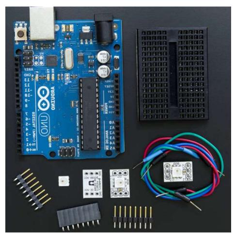
Inside the WS2812 and WS2812B packages resides an embedded version of the WS2811 constant-current LED driver, as well as 3 individually controlled LEDs; one red, one green, and one blue. In a compact package, the WS2811 includes:
