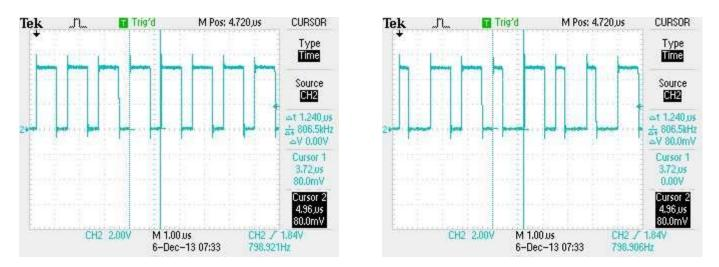
One of the advantages of using a microcontroller as opposed to, say a computer's CPU, is that we have a very tight control over the timing of the instructions we program into it. In fact, to show how precise that control can be, we'll be using assembly instructions instead of the typical high-level functions such as digitalWrite. The use of assembly allows us to know exactly how many clock cycles are taken up during the execution of each instruction.
