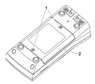
Place four batteries (type Mignon AA) in the battery compartment.
