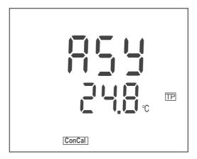
If necessary, set the temperature of the first buffer solution with <▲><▼>.
