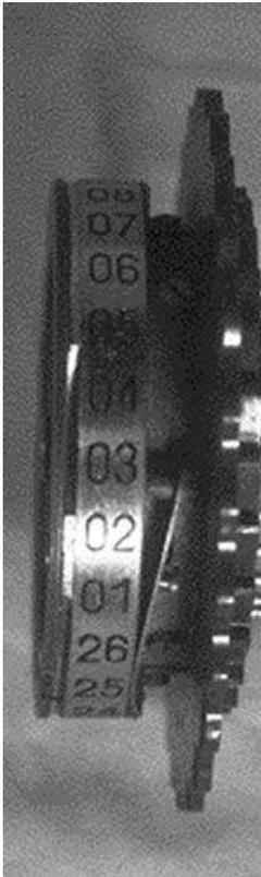
**Figure 4.11** An Enigma rotor.
