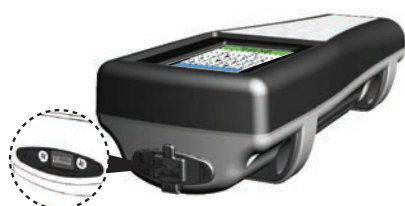
Figure 41 Micro USB female connector
