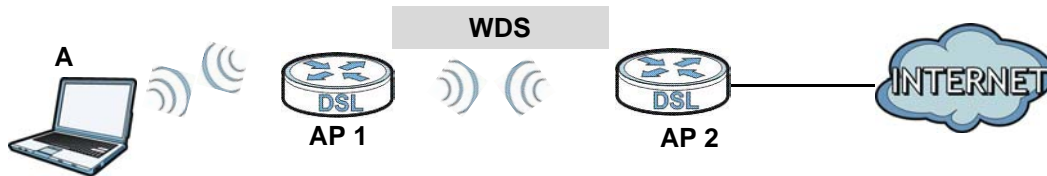
Figure 41 WDS Link Example
