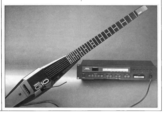
the G10 has a ninth velocity curve level that is not programmable and always sends a velocity of 1.
