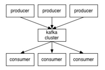
Kafka Brokers scale and perform well in part because Brokers are not responsible for keeping track of which messages have been consumed. Instead, the message consumer is responsible for this. This design feature eliminates the potential for back-pressure when consumers process messages at different rates.
