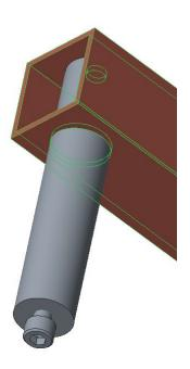
To create the pivot points for the intake arms, press the Igus plain bearings (in the Igus bag in the kit) into the ¾" holes you put in the intake arms. These should make for a low-friction and sturdy joint.
