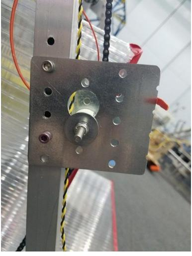
For the length of the chain run we just put together pieces of chain until it looked about right and then added a tensioner. There are better ways to do this such as calculating the center-to-center distance for the shafts however the VexPro Corner Gusset flexes making a chain tensioner necessary. Slide the assembled tensioner under the chain along the box tube until the chain is tight and match drill the holes for a 10-32 bolt, 1.5" long.
