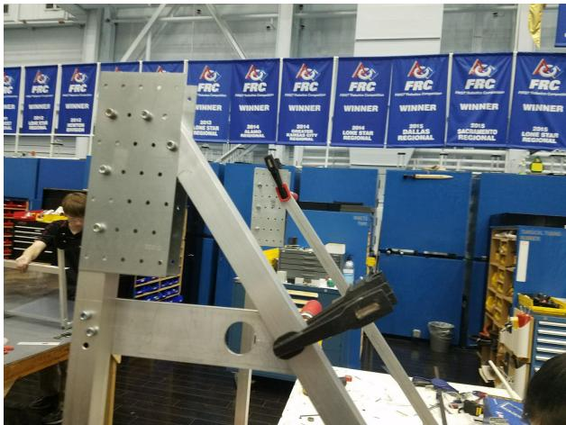
Next the ½" hex bearings can be placed into these bearing holes. The arm can also be placed in with the PVC Spacers. The 1.175" long spacer goes on the left and the 1.19" long spacer goes on the right when looking from the back of the robot. The ½" hex shaft is then pressed in, you may need to loosen the bolts on the Versahubs on the arm to get the shaft through all of them. Shaft collars then go on each end of the shaft.
