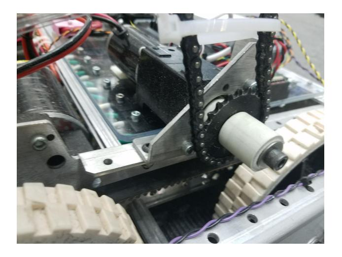
The chain tensioner consists of a tie plate cut in half with one of the holes drilled out to .86" A metric step drill is ideal for this, but it's ok if the hole is a little oversized. The other plate needs to have the hole directly across from the .86" hole drilled out for a 10-32 (.201") The following photos show how the tensioner is mounted with 10-32 bolts.
