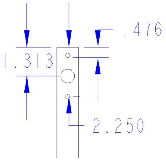
These are the only parts that need to be machined before being assembled. The rest will be clamped together and match drilled.
