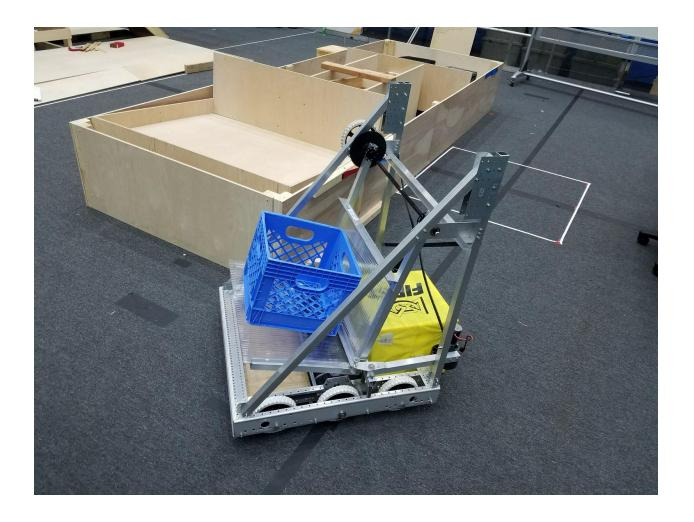
The last major thing to do for the arm is install the motor and the chain tensioner. Assemble a VersaPlanetary with a 100:1 and a BAG motor. Bolt the VersaFrame Corner Gusset in the location shown in the photo below with 10-32 button head bolts and then install the .10" long spacer closest to the motor followed by the 22 tooth sprocket followed by the 1.1" spacer then use a large \(^1/4\-20\) washer and bolt to retain the spacers on the shaft.
