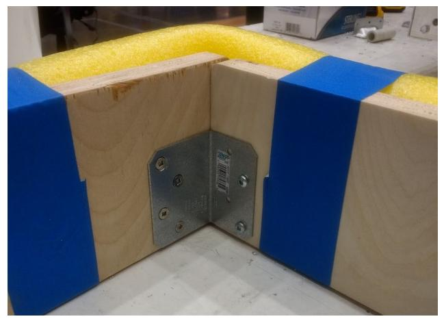
We used these steel gussets in the corners and attached them with wood screws. The two 4" long segments of angle mount the back of the bumper to the robot and the 2" long segments of angle attach the front of the bumper to the robot. Wood screws are used to attach the angle to the bumpers and then 10-32 bolts are used to attach the angle to the robot. The following pictures show an example of this.
