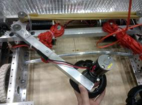
To start the match, the rollers are folded in towards each other and a zip tie is put loosely around the BAG motors. This loop is attached to the arm so that when it lifts, the intake flips outward, extending past the frame perimeter above the bumpers.
