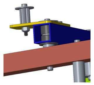
The final part you need to fabricate is from the leftover 1/8" plate from the front section of the AM14U chassis. Just cut a flat section from the C-channel and measure measure out these dimensions. This is the yellow part in the pictures above. The positions of the holes are the only critical dimensions, not the shape of the part.
