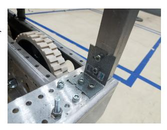
After the vertical box tubes are installed the tie plates can be clamped to either side of the 1x1s at the top. They need to be match drilled for a 10-32 bolt (.201") 1.5" long bolts need to be used to attach these components. If desired you can mark them and trim them to make them match the box tubes. Once the tie plates are installed the the two 41.5" 1" x 1" box tubes can be installed to
