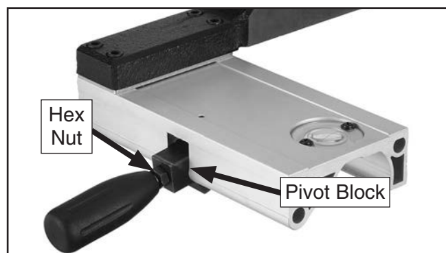
Figure 25. Handle installed on fence assembly.
