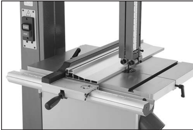
Figure 79. Resaw fence installed in the alternate position.
