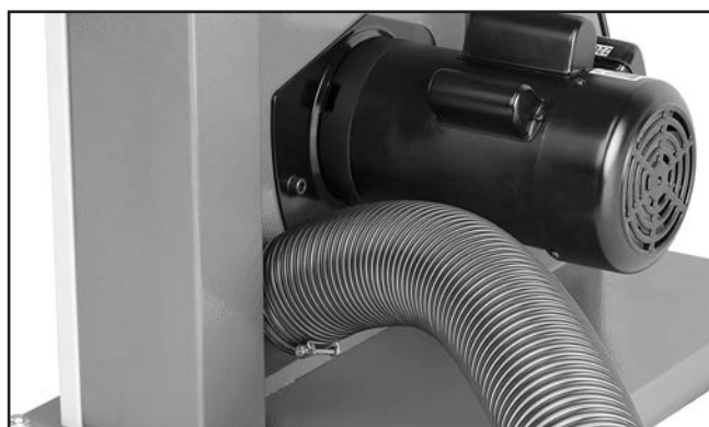
Figure 38. Dust hose attached to bottom dust port.
