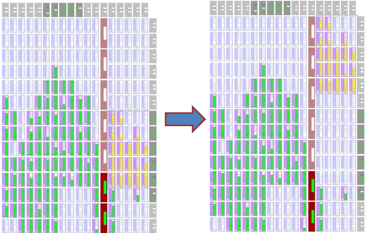
Figure 7-13: Moving a group of Logic Cells
