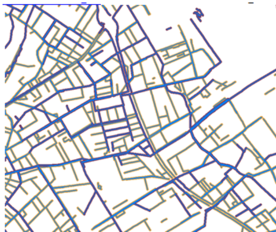
Example of an ISG capturing the combined primary and secondary surface water systems
