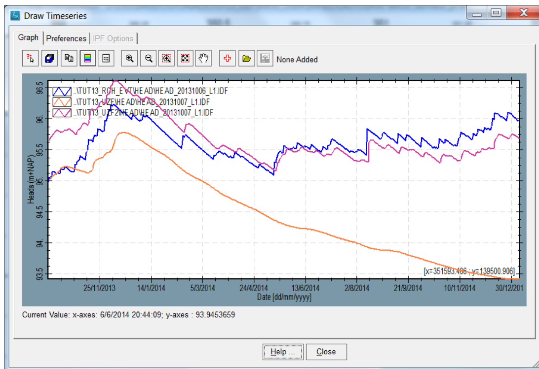
Figure 11.143: Time Series of computed groundwater levels for the combination RCH-EVT and the two variants with the UZF package.
