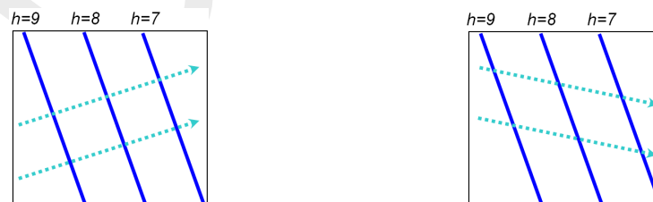
(a) Isotropic conditions, flow [q] perpendicular to piezometric head [h] (b) Anisotropic conditions, flow [q] non perpendicular to piezometric head [h]
