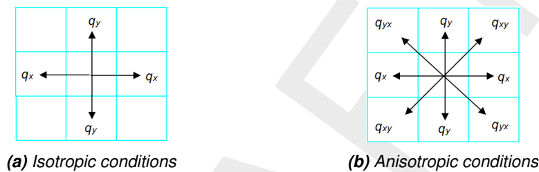
Figure 12.9: Example of (a) flow terms in isotropic flow conditions and (b) flow terms in anisotropic flow conditions.
