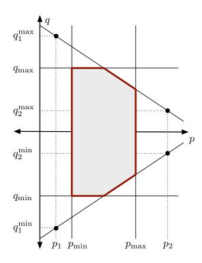
Figure 5-6: Generator *P-Q* Capability Curve
