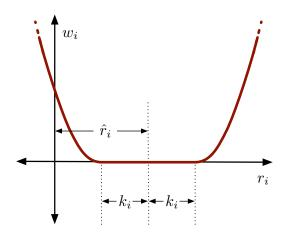
Figure 5-2: Relationship of  $w_i$  to  $r_i$  for  $d_i = 2$  (quadratic option)
