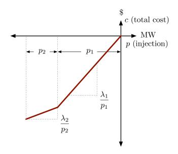
Figure 5-5: Total Cost Function for Negative Injection
