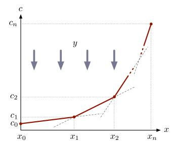
Figure 6-3: Constrained Cost Variable
