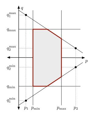
Figure 6-6: Generator *P*-*Q* Capability Curve
