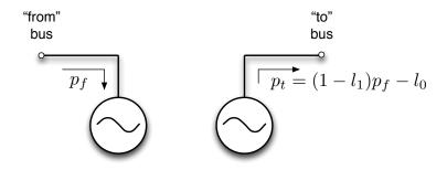
Figure 7-3: Equivalent "Dummy" Generators
