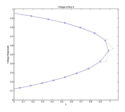
Figure 5-1: Nose Curve of Voltage Magnitude at Bus 9
