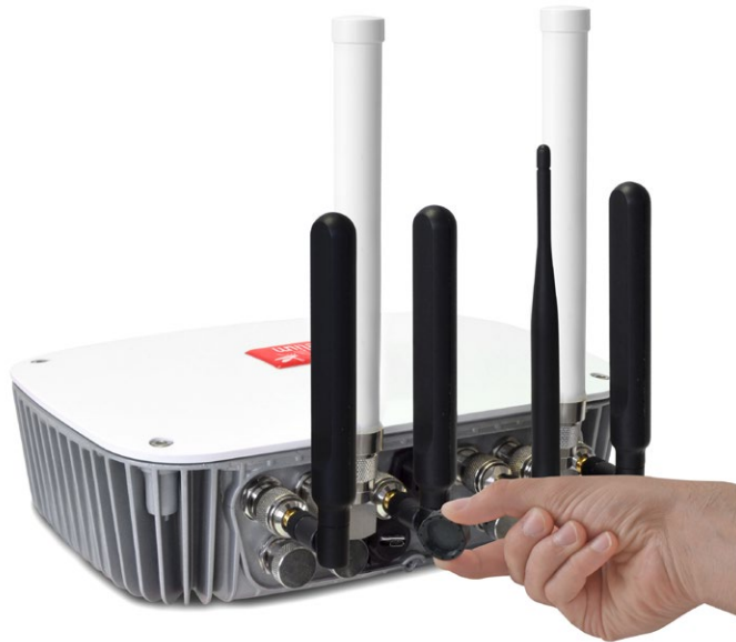
Figure: External SIM socket in a Meshlium with 4G/3G/GPRS/GSM module
