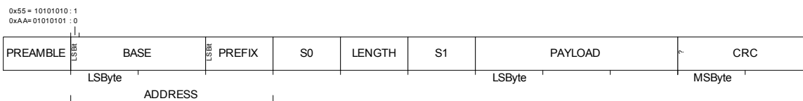
Figure 19 On-air packet layout
