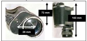
offset between the optical axis of the objective and the optical axis of the eyepiece is 28 mm.
