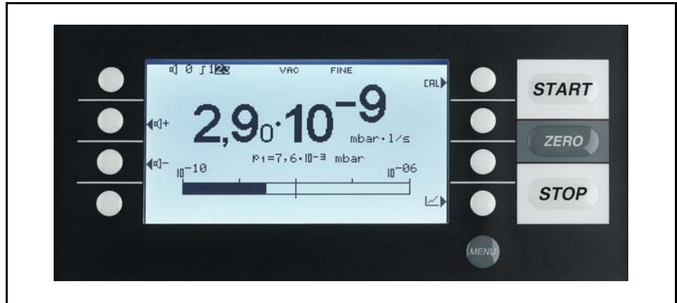
Fig. 10 Display: Measurement mode with bargraph
