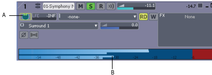
A. Micro surround panner in Track view B. Six channel output meter
