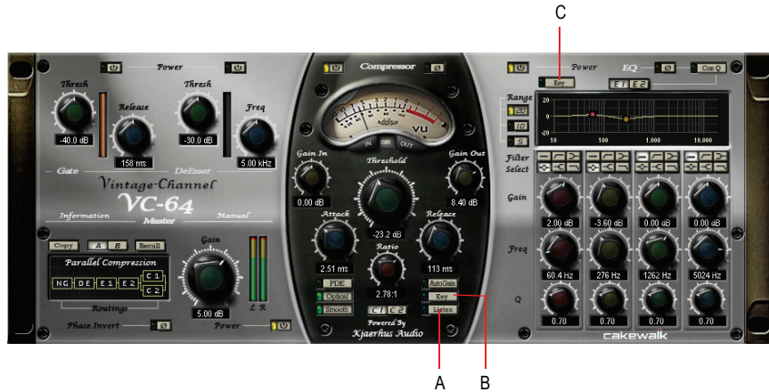
A. Sidechain Listen B. Enable/disable sidechaining for the current Compressor C. Enable/disable sidechaining for the current EQ
