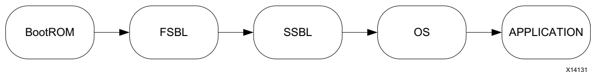
Figure 3-1: Typical Boot Flow
