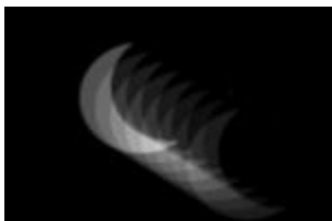
Motion blur without supersampling—multiple exposures are visible
