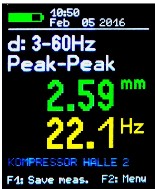
Figure 7: Battery indicator upper left
