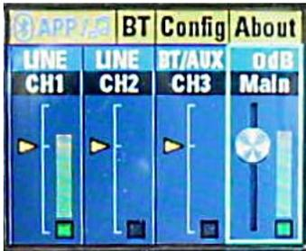
Fig. A Level Indicator Bars
