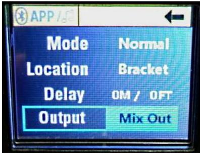
**Fig. 30** Output Parameter, Mix Out Selected
