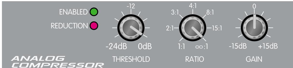
Limiting at maximum level. Can be used to avoid digital clipping.
