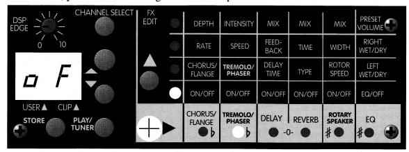
When the LED below the effect you wish to edit lights, you'll notice that the display reads either **on** or **of** (off). This corresponds to whether or not the effect is currently in use or not. To change this parameter, use the parameter  $\triangle$  or  $\nabla$  buttons.
