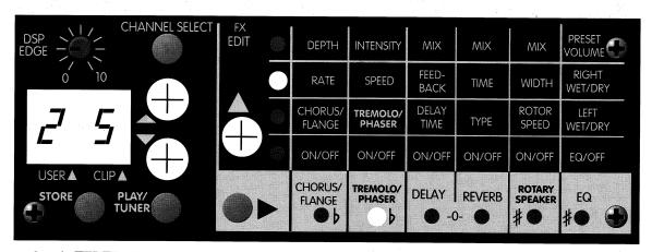
Now use the  $\triangle$  **FX EDIT** button again to select the intensity parameter and use the parameter  $\triangle$  or  $\nabla$  buttons to set it to 85.
