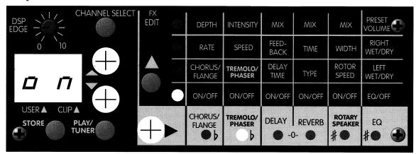
Now, using the  $\triangle$  **FX EDIT** button, step through the various editable parameters of the particular effect you're adjusting. When the LED lights in the same row as the parameter that you wish to edit, use the parameter  $\triangle$  or  $\nabla$  buttons to change it to your desired setting.
