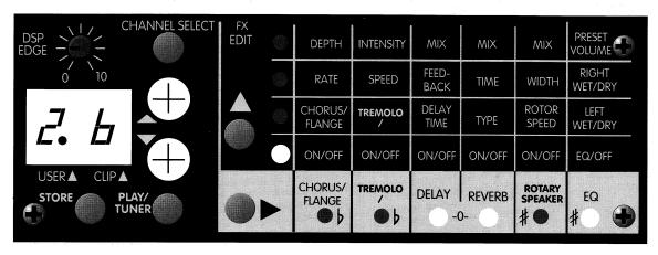
Select the effect you wish to add, delete, or edit using the ►FX EDIT button. As the FX EDIT buttons are pressed, the vertical column of LEDs will show which parameter is being edited, while the lower row of LEDs will show which effect is being edited. As you scroll through the various effects, the main LED display will indicate whether the effect is "on" or "of" (off). Use the parameter ▲ or ▼ buttons to turn the tremolo effect on.
