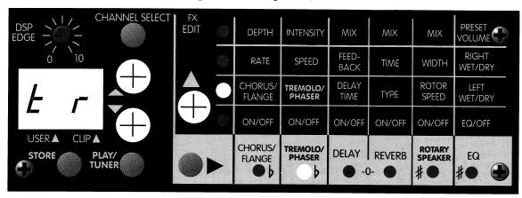
Now use the  $\triangle$  **FX EDIT** button again to select the speed parameter and use the parameter  $\triangle$  or  $\nabla$  buttons to set it to 25. Note that if the parameter  $\triangle$  or  $\nabla$  button is held down, it will scroll to the desired value.
