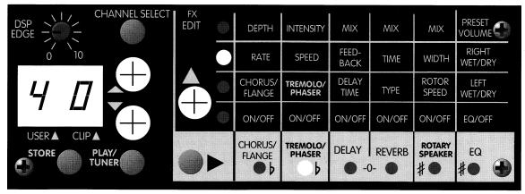
To store your newly created guitar tone, press the **Store** button. The display will start to flash, and will indicate the target storage location. You can either use the parameter  $\triangle$  or  $\nabla$  buttons to change the preset target location, or just hit **Store** again to save to the current preset location. That's it.
