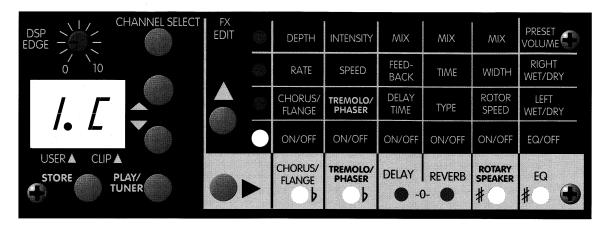
This particular display indicates the amp is set to User patch 1.C, and the following effects are active: Chorus/Flange, Tremolo/Phaser, Rotary Speaker, and EQ.
