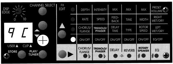
The preset that is active now should be **9C** the last factory preset. This preset is set on the Clean channel and contains no effects, so you can adjust the Clean channel to your particular taste.
