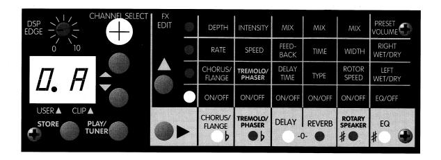
At any time, the **Channel Select** button can be used to change the selected preamp channel from Clean to Lead, or vice versa. This can be very useful when trying patches in different modes. If you change to the next preset without storing this change, the channel selection change you made will simply be ignored.
