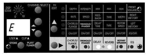
Since the tuner is a full chromatic tuner rather than dedicated to EADGBE tuning, you can detune the whole instrument simply by tuning to whatever notes you desire (for example, you could tune down 1/2 step to Eb-EbAbDbGbBbEb, open A tuning — EAEAC#E, drop D tuning — DADGBE, etc.)
