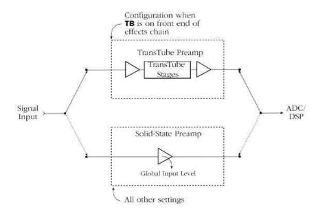
Note: The Global Input Level is non-functional when the Transtube (TB) is at the front of the effects chain.
