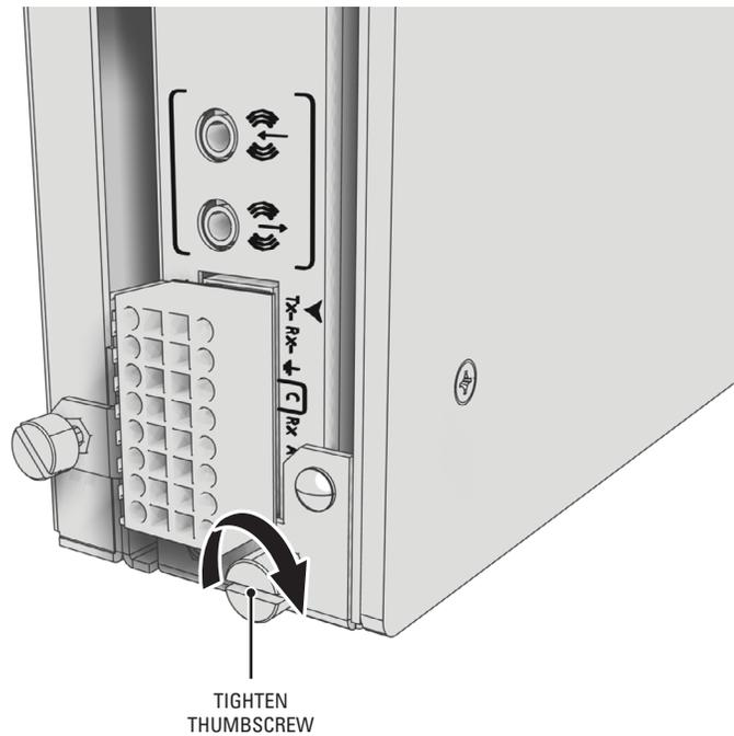
**Figure 7.** Tighten the Thumbscrew to Secure the Unit
