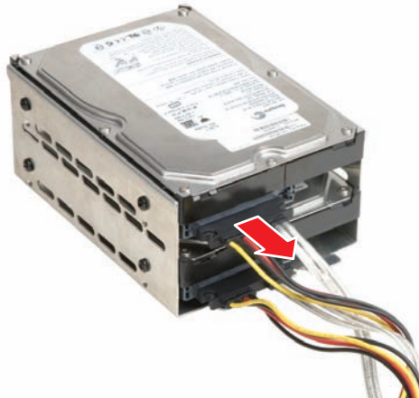
Figure 6. Removing the Power and Data Cables
